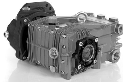
Figure.16 - Checking Pump and Gearbox Oil Level
