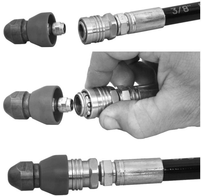
Figure.9 - Nozzle Quick Connect Operation
