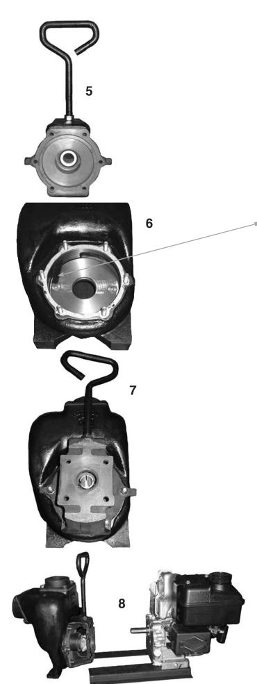
5. Remove the white ceramic seal and rubber cup from the rear adapter. Clean the recess opening with sandpaper or wire brush.
