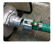
Fit camlocks to pump (thread tape here) and hose
