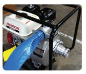
Connect layflat with pump coupling supplied with pump
